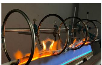
The cable is exposed for 15 minutes to flame at 650°C and for additional 15 minutes to fire and water spray.
